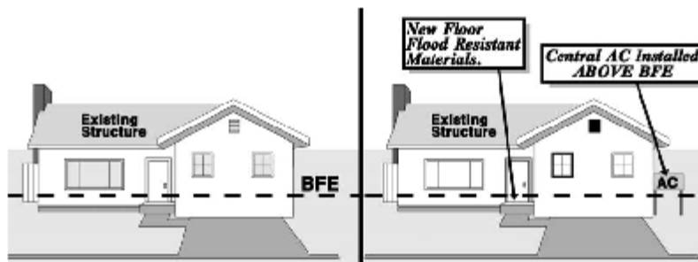
Figure 8-2. Minor rehabilitations use flood-resistant methods and materials
